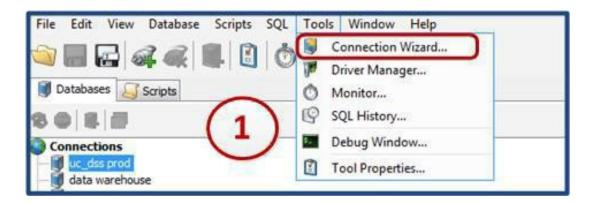
The connection wizard will guide you through the steps to set up a database connection. Enter a <u>Connection Alias</u> for the database you are attempting to set up a connection to. Click on the <u>Next</u> button.
